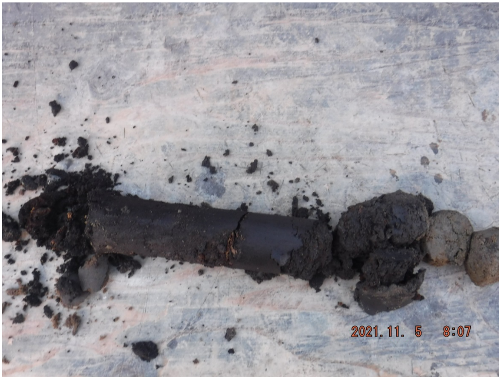
Photograph 4: Buried topsoil, BH21-3 at a depth between 5.4 and 6 m
